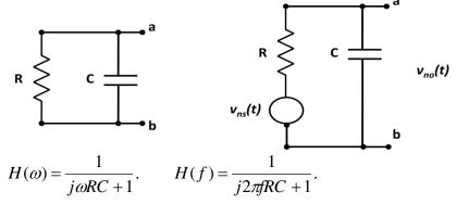
The power density at the output terminals is  $P_o(f)$  given by
